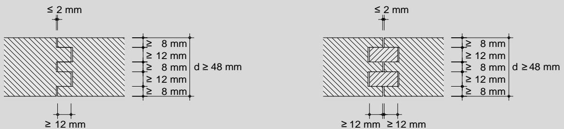
**Typ 3: Nut und Kamm/Feder**
